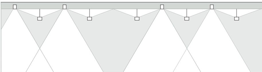
Suspended light structure with indirect luminaires for fluorescent lamps.
