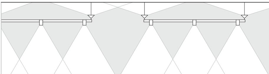
Light structure with uplights designed for compact fluorescent lamps, downlights for halogen lamps, and track-mounted spotlights.
